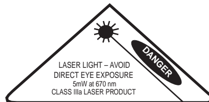
SA1M Laser Mark Sensor: Class IIIa Laser (670nm) Visible Beam
