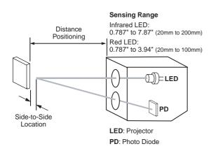
The photoelectric position sensor projects a beam from an LED, through the projection lens, to the object. Units are available with infrared or red LED. Reected light from the object is collected by a photo diode.
