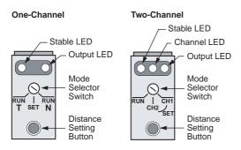
**Mode selector switch:** Select SET to memorize position distance, RUN N to operate in normal mode, or RUN T to operate in tilt mode. Tilt mode is recommended for the precise detection of an object's leading edge and for sensing objects with varying intensities of reected light (for example, dark objects together with light objects).
