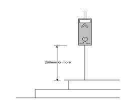
Detecting the presence of an object in front of an immediate background
